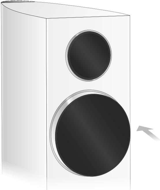
2. Turn it clockwise or counter-clockwise until you can feel the magnets attach to the screws below.
