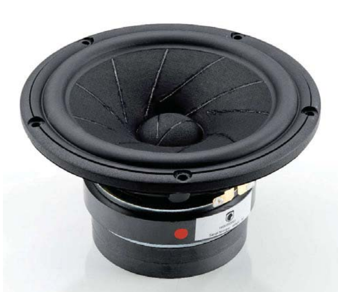
The woofer of FM-2 is built by Scan-Speak and customized for Gato Audio. Note the distinctive pattern of membrane reinforced with the “slice” of stiffer material and the double ferrite ring outside.
