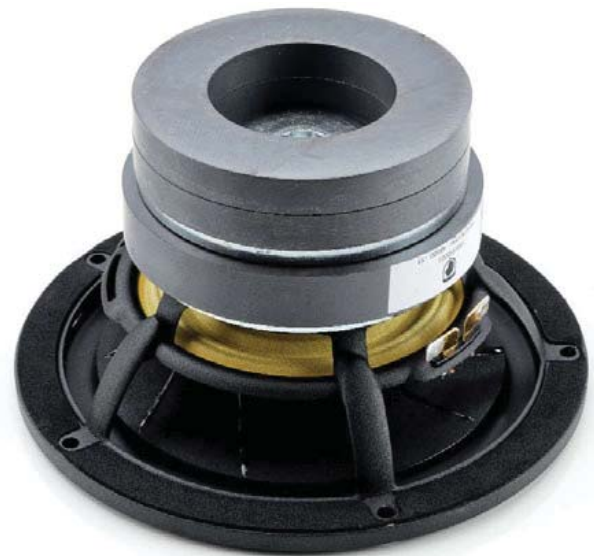
The woofer of FM-2 is built by Scan-Speak and customized for Gato Audio. Note the distinctive pattern of membrane reinforced with the “slice” of stiffer material and the double ferrite ring outside.
